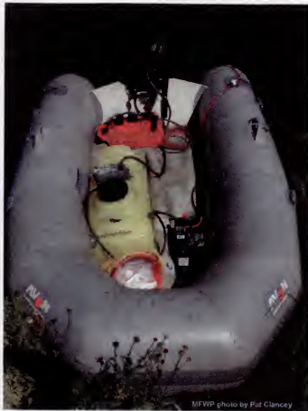
Figure 15. Inflatable raft set-up used to apply Fintrol to Cherry Lake. Note the red dyed liquid in the tubing on the port side of the raft.
